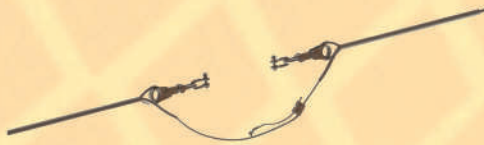
OPGW Double Tension Assembly (Passing Through Type)
